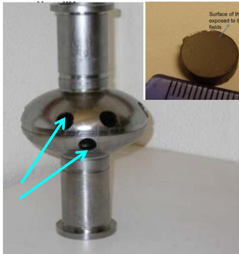
Samples cut out from processed and tested cavity
